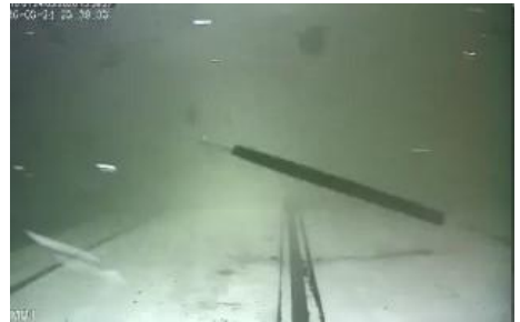
Right: a metal cylinder "fake fish" is passed through the counter on a line to confirm sensitivity.
